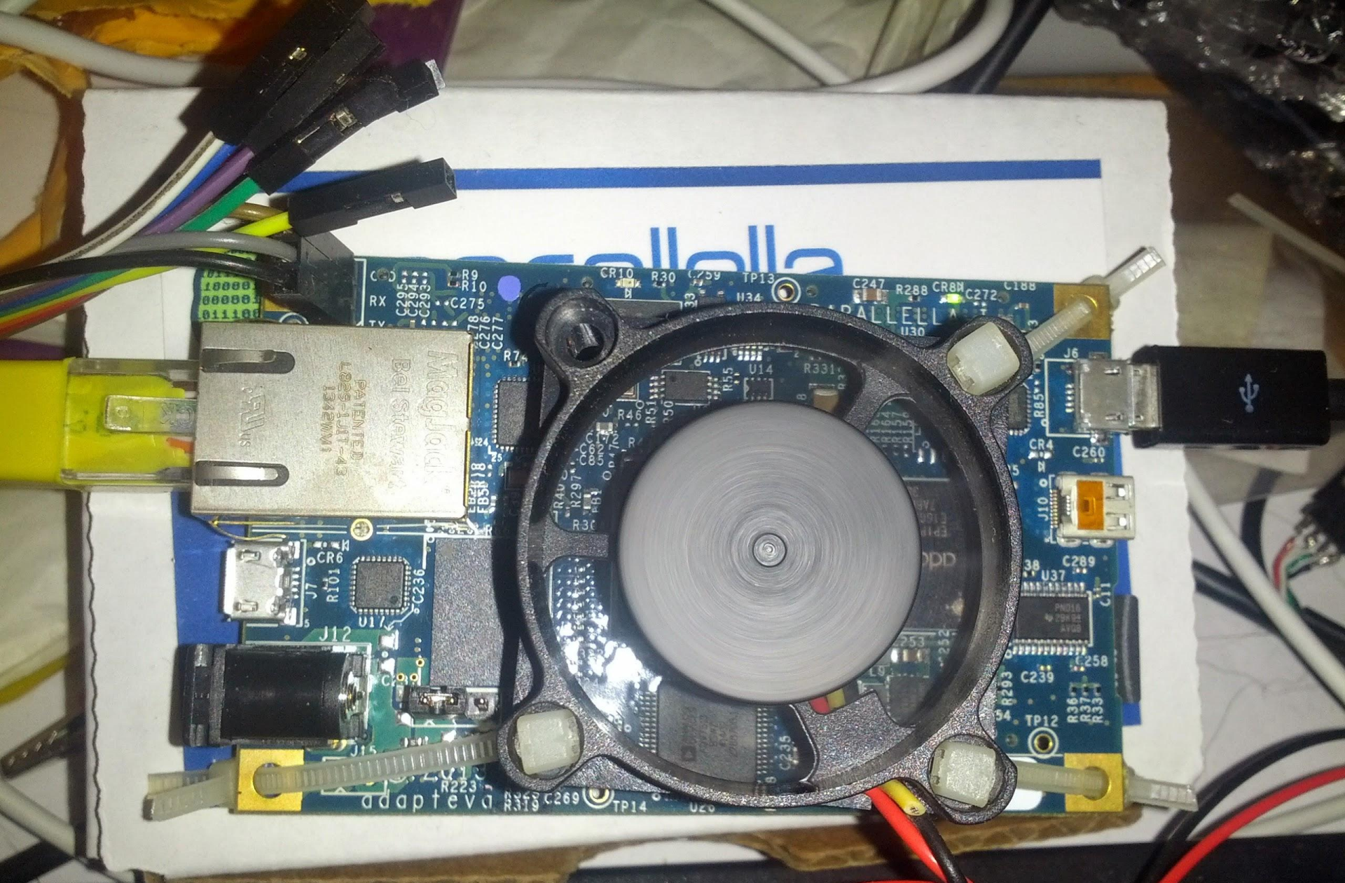
18 months later... with extra heatsink, but still requires some airflow :-)
