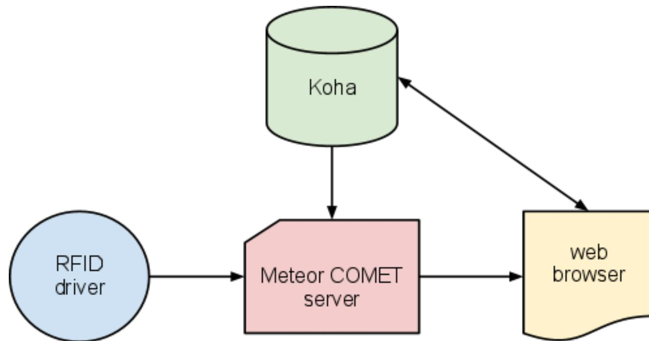
Meteor Comet server: single point of failure
